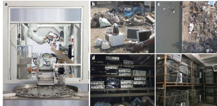
Fig. 1 | Approaches to electronic waste dismantling. a–e, There is a marked difference between formal e-waste dismantling, such as Apple's Daisy robot (a), and manual dismantling, such as that in the Agbogbloshie market sector in Accra, Ghana (b). Informal e-waste resource recovery leads to environmental pollution (c), while stockpiles of e-waste awaiting recycling in government-approved facilities on the outskirts of Beijing, China, continue to grow (d,e), requiring urgent solutions. Credit: photograph in panel a courtesy of Apple, Inc.; photographs in panels b–e taken on location by O.A.O.
